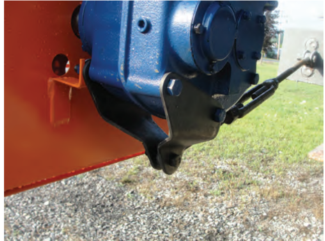
Torque Arm Included With Shaft Mount Reducer
