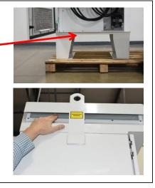
4. Inspect tunnel internally for blockage, through access panels located on front of tunnel above and below VFD. Remove any blockages.
