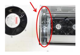
5. Inspect necessary and clean front door air filter (use warm water; dry filter before re-installing). Replace when.
