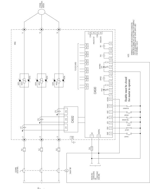
**10.5 THREE WIRE CONTROL WITH SHORTED SCR DETECTION**
